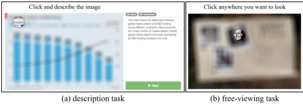
Fig. 2. Two different versions of the BubbleView interface for two task types, for gathering task-based (a) and task-free (b) clicks, as approximations to similar eye tracking experiments.
